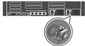
**4** Loop and secure the power cable using the retention strap.
